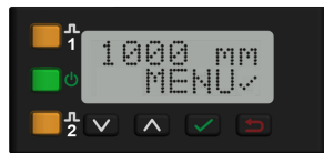
Figure 2. LE550 Display in Run Mode
