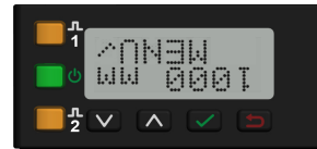
Figure 23. LE550 Inverted Display Orientation
